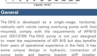
some unique design in hydraulic, connection of pump body and bearing bracket, stiff impeller, mechanic seal cooling system and auxiliary system. The HP –OH2 pumps modular construction system offers wide ran ging interchangeability of components such as shafts, casing s, covers, wear rings, shaft seals and bearings among the various pump ranges.
